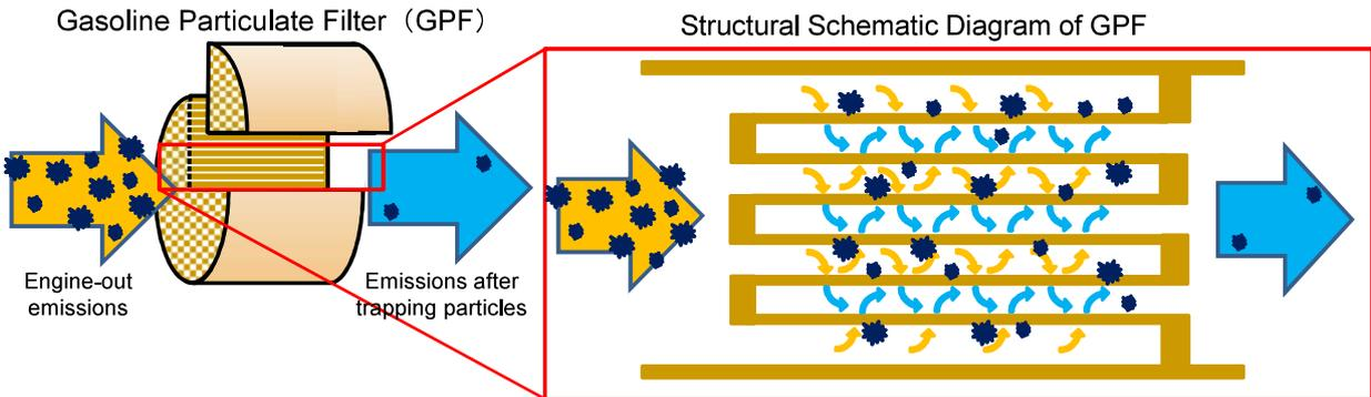
\*The combustion temperature of gasoline vehicles is higher than that of diesel vehicles. Therefore, when PM is accumulated in the filter, natural regeneration occurs by burning PM during fuel cut due to deceleration. However, additional measures are necessary when the temperature required for PM combustion is not achieved or when sufficient amount of oxygen is not secured for combustion, such as during continuous low-speed driving.
